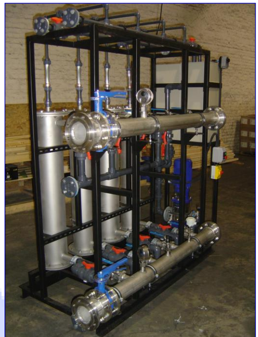
8" UF RIG INCLUDING CLEAN IN PLACE SYSTEM
