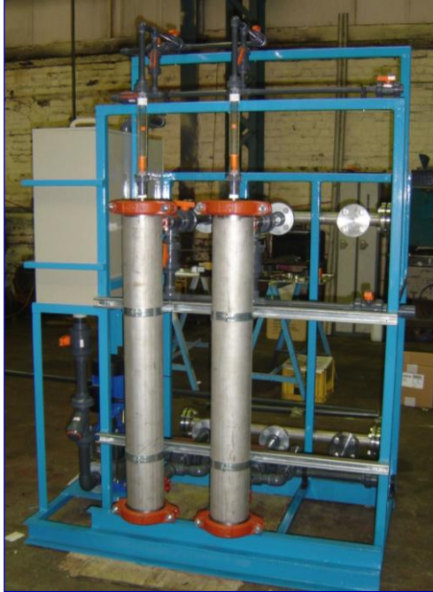
6" UF RIG INCLUDING CLEAN IN PLACE SYSTEM 600ltr/hr PERMEATE
